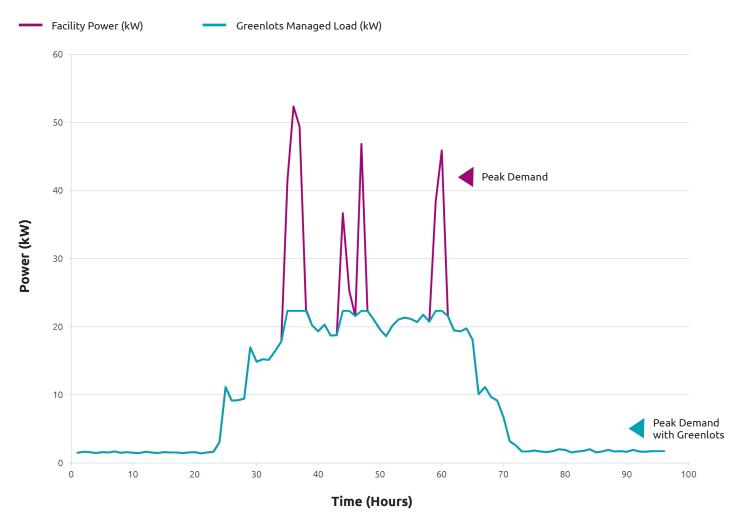
To prevent overload of our current electrical power infrastructure, energy demand from electric vehicle charging needs to be managed
